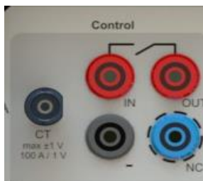
Connection input of current clamp for coil current reading on TM1700.
